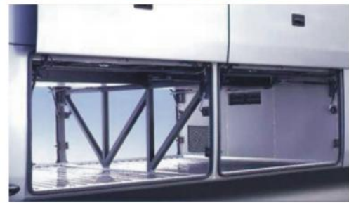
The super-large thru type luggage compartment eases the access of luggage.
