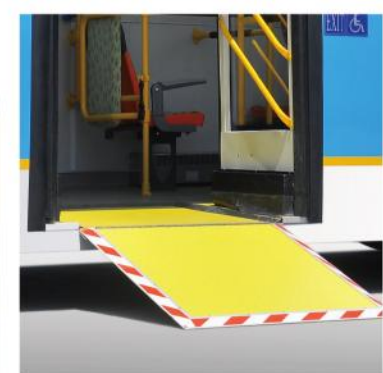
The reasonably arranged standing posts, handrails, and ring handles provide a better safety guarantee for the passengers. The ultra-low floor and single-stage footplate design ease the access of the passengers.
