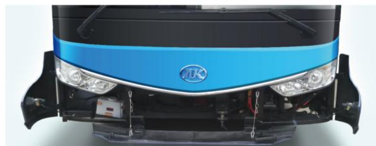
Openable front face design .The front face can be opened in four directions for the ease of repair and maintenance.
