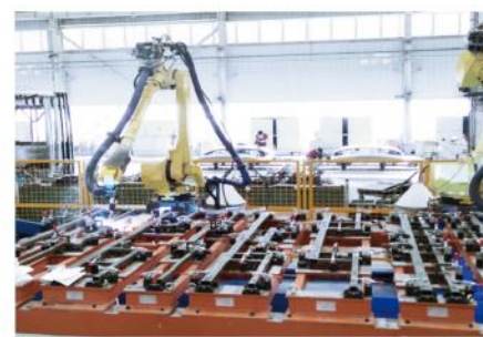
Robot welding for small assemblies
